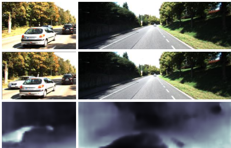
Fig. 4. Some failure cases of our method on KITTI. First column is a detail of a larger image. The foreground car is moving forward and it's detected as far away, while the background car is moving toward us and is detected as close. Second column is a poorly textured road.
