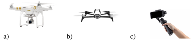
Figure 1. Camera stabilization can be done via a) mechanic gimbal or b) dynamic cropping from fish-eye camera, for drones or c) hand-held cameras
